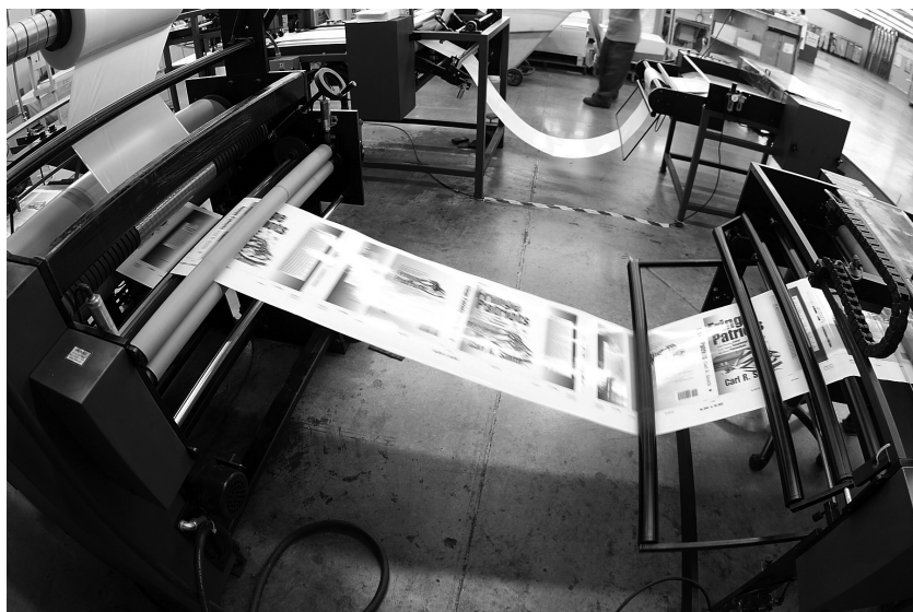
Four-colour book jackets being laminated at Lightning Source
